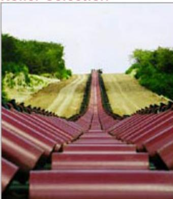
The loading capacity of a roller is determined by the bearing size, the axle diameter and the thickness of the shell.
