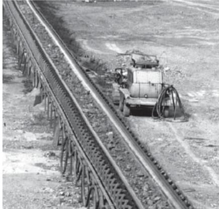
The residual material remains attached to the return section of the belt and may deposit onto the rollers in a non uniform way that promotes belt drifting and premature wear.
